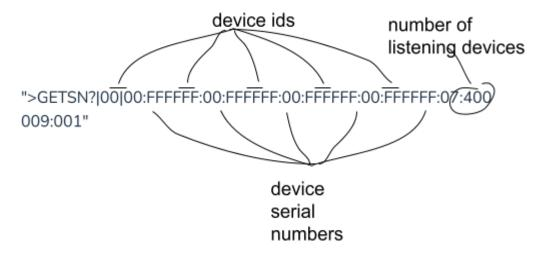
In the example above, only 1 Pressure Controller is connected to the Control Center.
